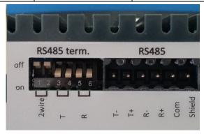
Example of DIP-switch settings. 4-wire with termination
