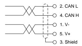
For reliable fieldbus function, line termination must be arranged in both ends of the transmission line. For a G5 Instrument placed at the end of the line, terminate line by placing a 121-ohm resistor between CAN L (pin 2) and CAN H (pin 4).
